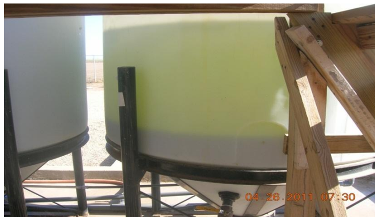
Figure 4. Flocculation drops algae out of suspension to the bottom and leaves supernatant at the top.
