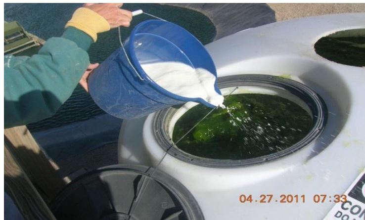
Figure 3. Addition of flocculation agent.
