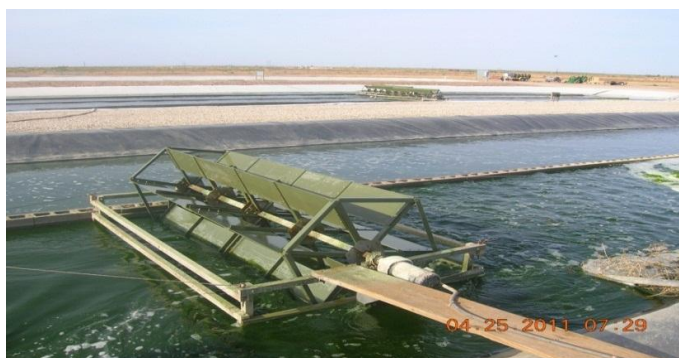
Figure 1. Twenty-five thousand gallon capacity raceway pond used during the demonstration. A 100,000 gallon capacity raceway can be seen in the background.
