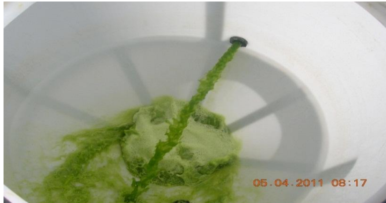
Figure 2. Cone-bottom tank into which pond culture was harvested.
